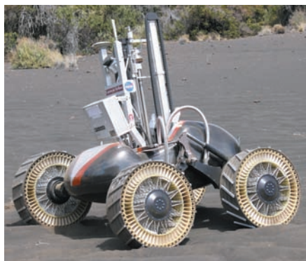
Fig. 3 — The Michelin Tweel is being considered for the wheels of the new NASA Lunar Rover.
